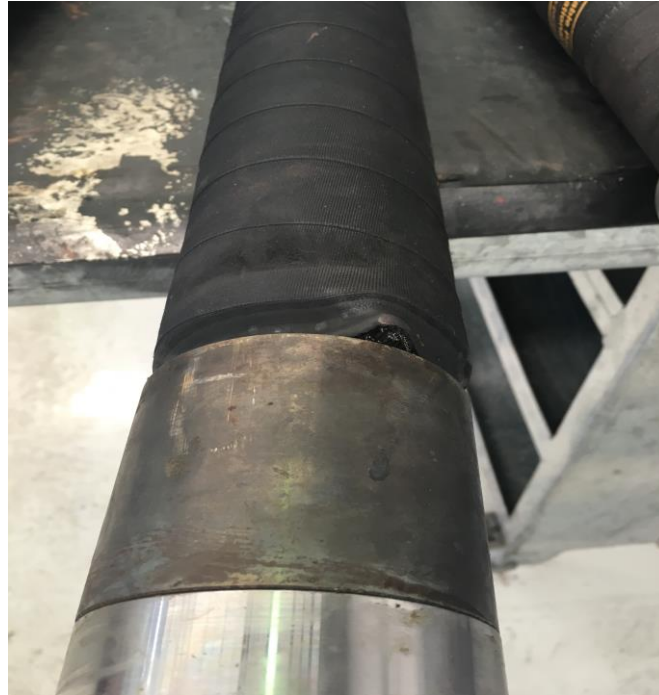
IPI Tubeless Construction Controlled Failure Mechanism Test after 150 cycles above 10,000 psi. Up to 3x expansion, full recovery.
