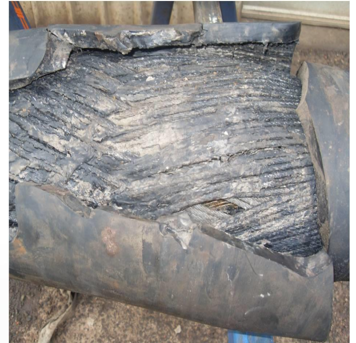
Cable/Wire Weave Element Construction. 5,000 psi / 2x max expansion, limited cycles with memory
