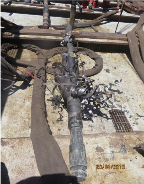
Slat Element Construction. Single set, up to 8,000 psi, 3x expansion, limited recovery
