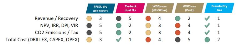
• <u>KEY TAKE AWAY</u>: PDG is a compelling development option for long, deep subsea tie-backs. Removing liquids from the pipeline along the route results in a significant reduction in both hydrostatic and frictional pressure drop without the use of large amounts of power
