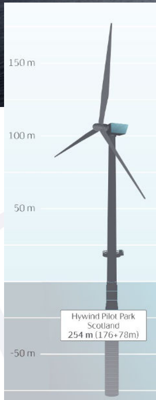
Spar Buoy: Hywind Scotland Pilot Park (5 x 6MW)
