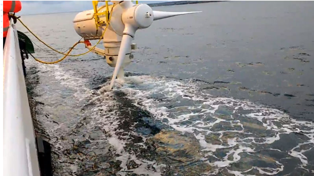
Flow past stationary turbine during recovery
