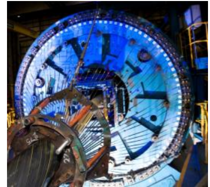
Application of Tensile Armour
