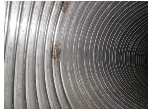
T-Strip in Carcass (Source: GE Oil&Gas)
